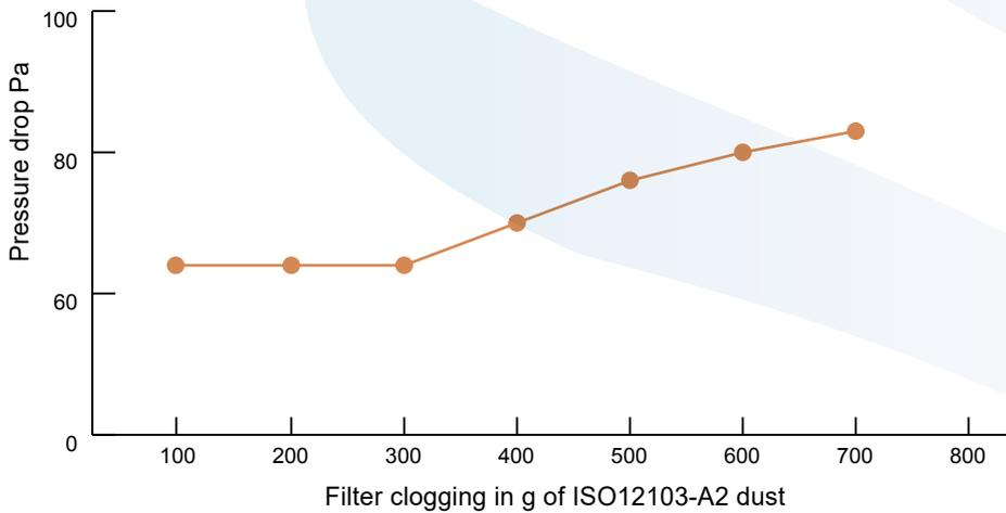
**Test performed at 3400 m<sup>3</sup>/h - Speed air passage 4m/s**
